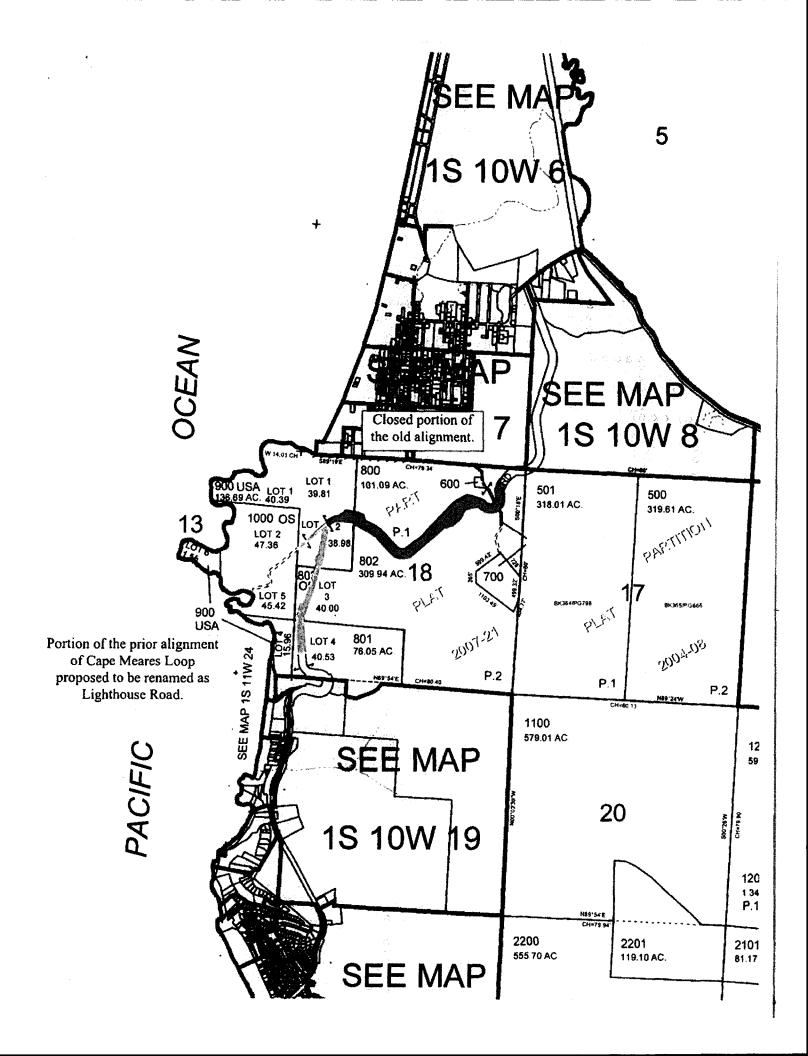
Closed portion of the old alignment. Portion of the prior alignment of Cape Meares Loop proposed to be renamed as Lighthouse Road. New alignment of Cape Meares Loop. Google Earth
