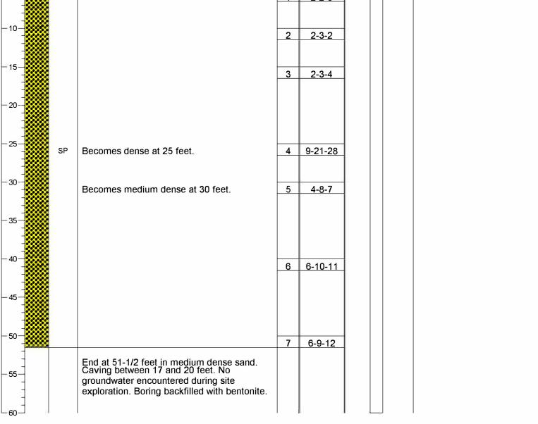
BORING METHOD: SS ELEVATION REFERENCE: START CARD/TAG ID:
